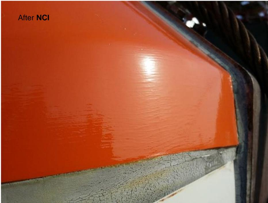
The weather did not allow for the NCI to level as it normally would however plenty of material was applied to the surface of the lifeboat to achieve the target dry coating thickness of 1+ mils that will provide for long term protection.
